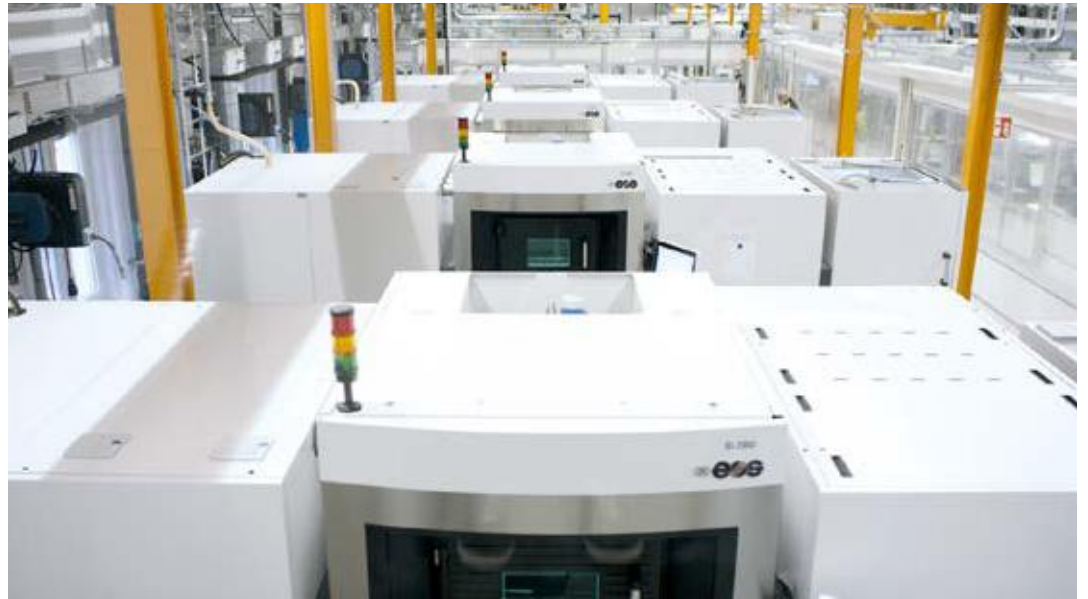
The additive manufacturing shop floor in Finspång, Sweden, where Siemens builds gas turbines for power plants using industrial 3D printing technology by EOS.
