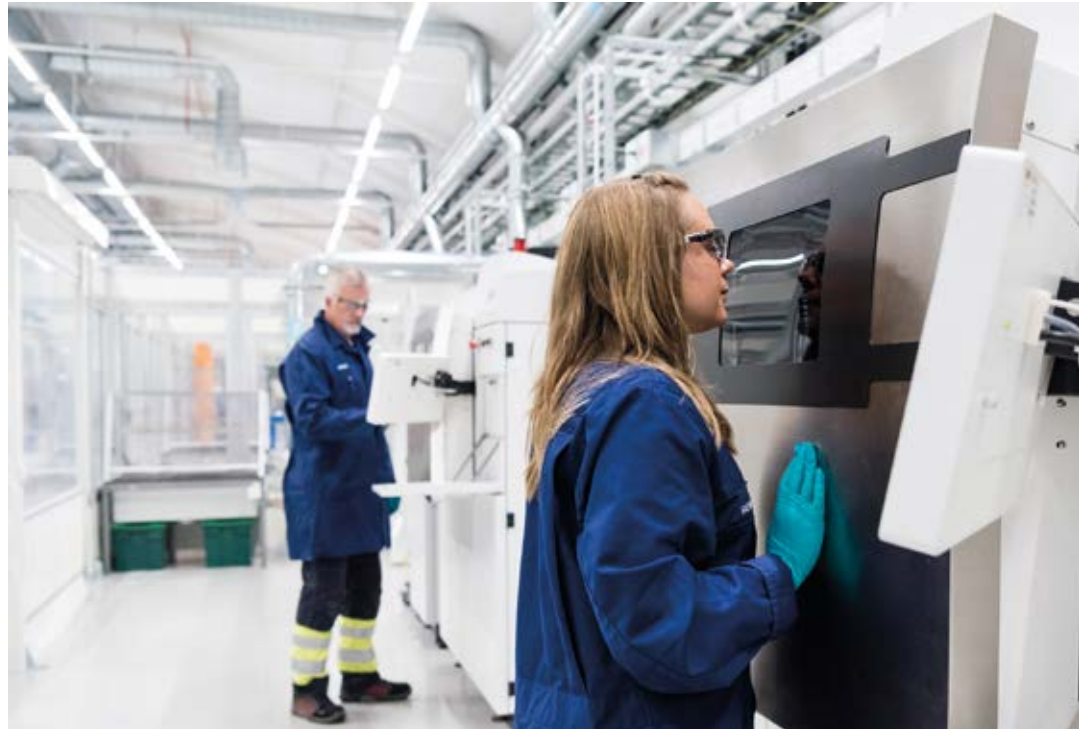
A look at the 3D printing shop floor at Siemens, in the Swedish town of Finspång – producing in series metal parts with additive manufacturing (Source: Siemens).
